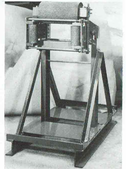
ABOVE: Producing a 'rustic' texture on the clay column.
