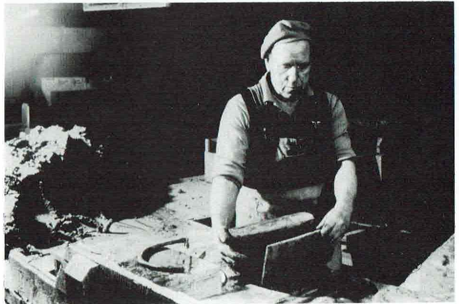
The sequence of hand-moulding. ABOVE: Cutting off the excess clay with a wire bow. BELOW: The full mould is lifted off the stock board and the brick turned out on to a pallet.
