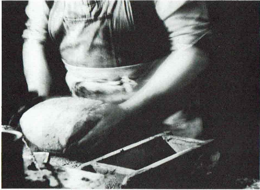
The sequence of hand-moulding. ABOVE: Forming the clot by rolling it in dry sand on the bench. BELOW: Throwing the clot into the mould. Standard-sized brick moulds are of hardwood lined with steel, though plastics are now being introduced. Moulds for specials are of wood.
