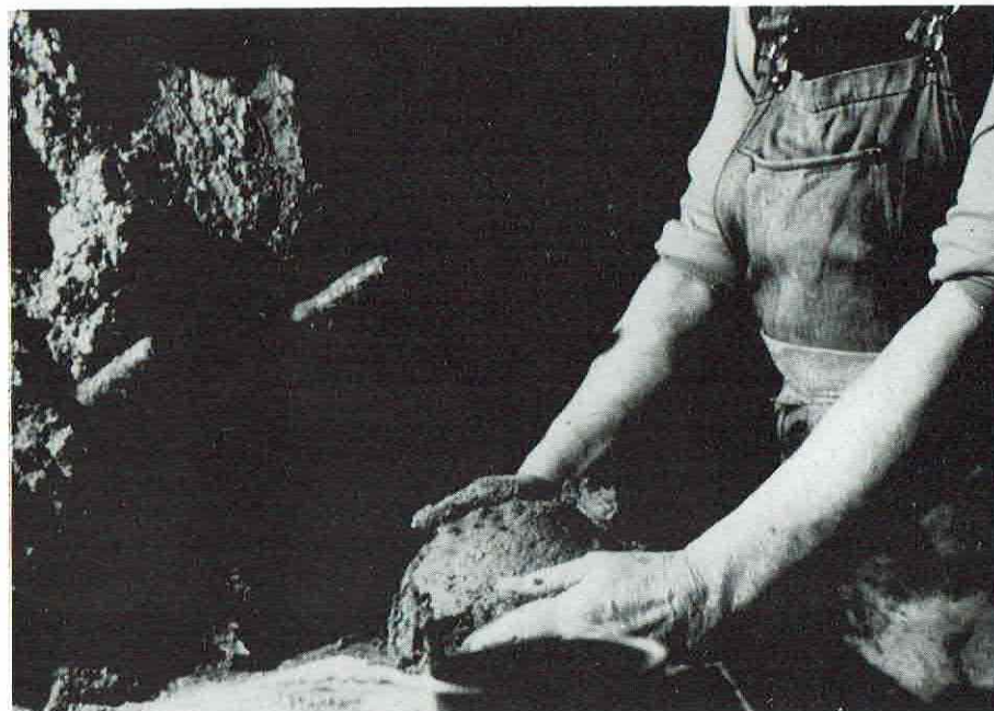
The sequence of hand-moulding. Taking clay from the heap on the bench, using a two-handed 'cuckle'.
