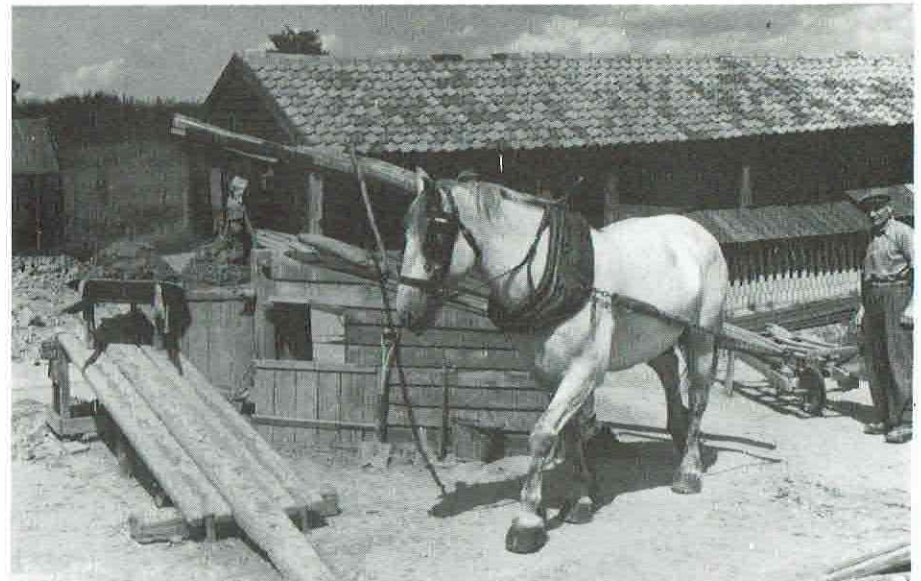
Horse-operated pugmill, South Cove, Suffolk. Beyond the mill, bricks are drying in hacks under a permanent tiled roof and movable wooden caps. In front of the man is a hack barrow for transporting freshly made bricks to the hacks.
