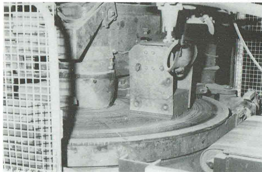
Pressing calcium silicate bricks, three at a time, in a rotary-table type press.
