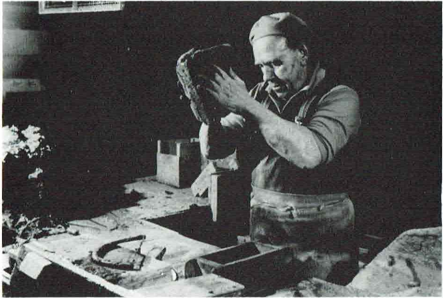
The sequence of hand-moulding. ABOVE: Forming the clot by rolling it in dry sand on the bench. BELOW: Throwing the clot into the mould. Standard-sized brick moulds are of hardwood lined with steel, though plastics are now being introduced. Moulds for specials are of wood.
